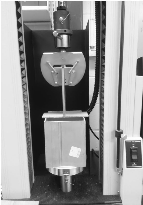
Heirloom composite material loaded into the testing machine
