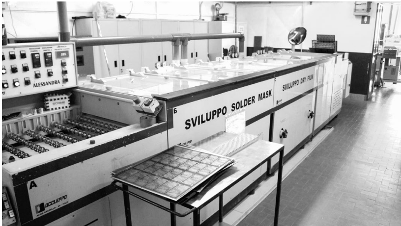
The machine that develops the photoresist
