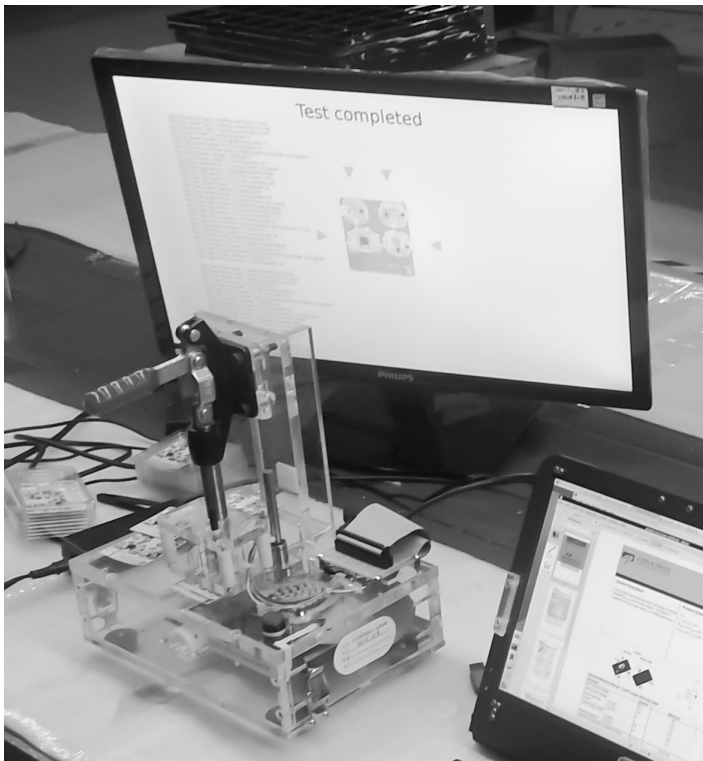
The testing machine for the Chibitronics microcontroller sticker
