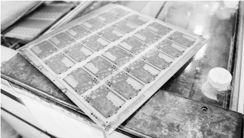
A panel etched of unwanted copper
