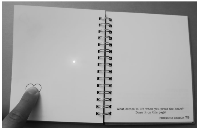
The DIY pressure sensor with paper overlay
